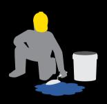
Compact the product by tapping with the back of the shovel or with a drum, vibrating plate or repeatedly pressing the wheel of a car
