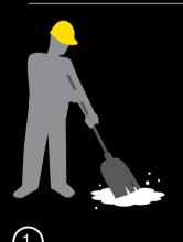
Clean the pit from any remainings and remove all loose pieces around the hole
